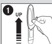
Slide hook up to remove from mounting base.
