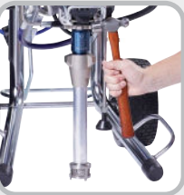
Loosen the Clamping Nut
