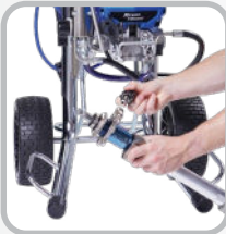
Remove Hose & Suction Tube
